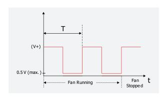
Open Collector Tachometer "FG" output voltage waveforms
