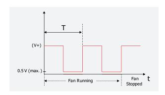
Open Collector Tachometer "FG" output voltage waveforms
