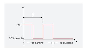
**Tacho Frequency** RPM=60/2T=30 f (f=frequency)
