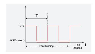
Open Collector Tachometer "FG" output voltage waveforms
