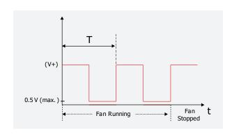
Open Collector Tachometer "FG" output voltage waveforms
