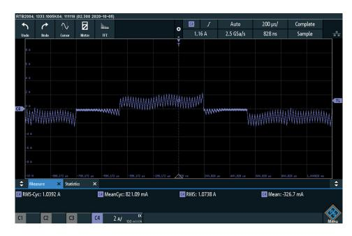
Figure 2: Phase Current With Motor Choke
