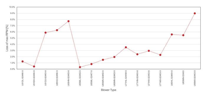
Figure 4: Loss of Max. RPM with Motor Choke
