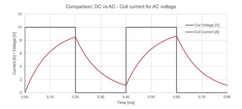
Figure 6: Current Behaviour Depending on Voltage Form
