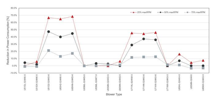
Figure 3: Reduction in Power Consumption With MCM-33/10
