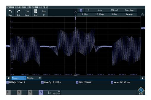
Figure 1: Phase Current Without Motor Choke
