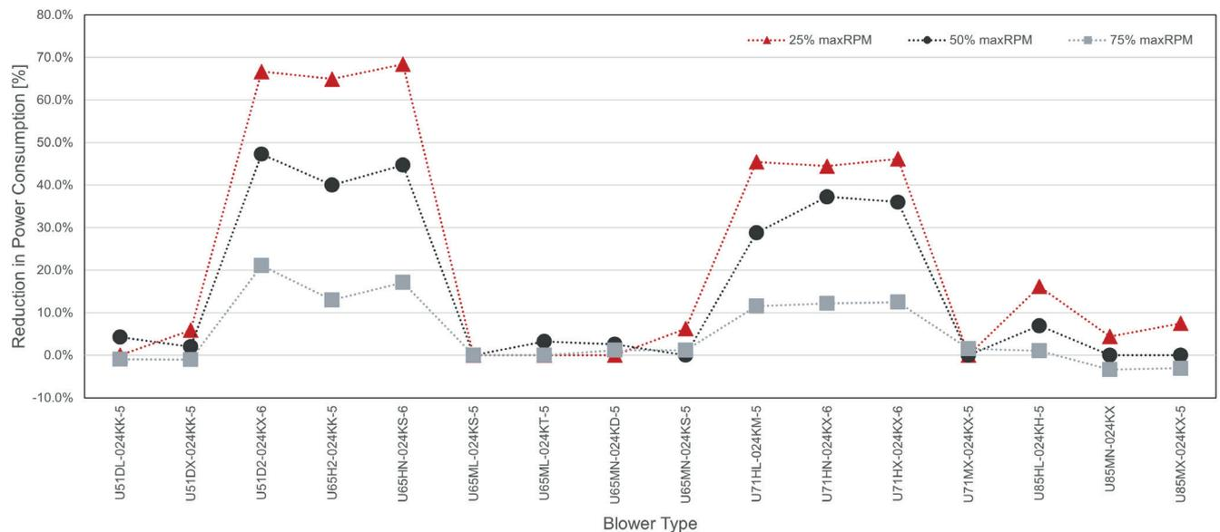
Figure 3: Reduction in Power Consumption With MCM-33/10
