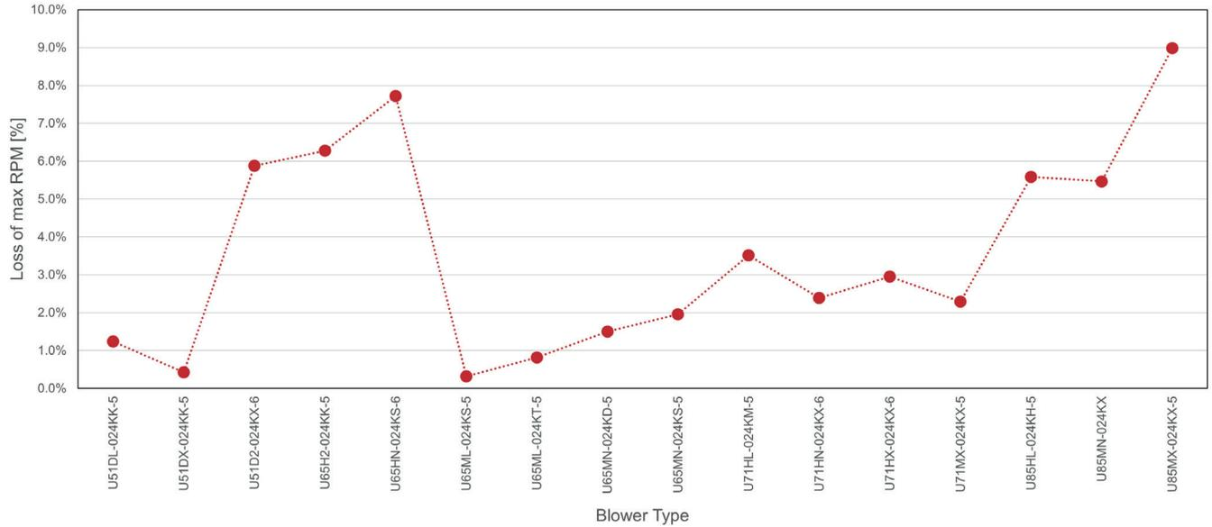
Figure 4: Loss of Max. RPM with Motor Choke
