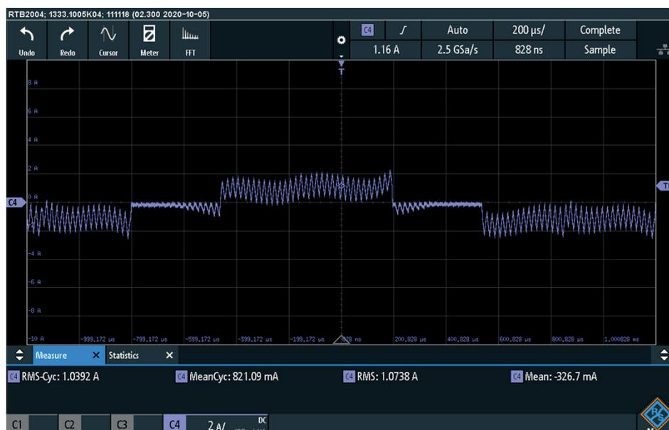
Figure 2: Phase Current With Motor Choke
