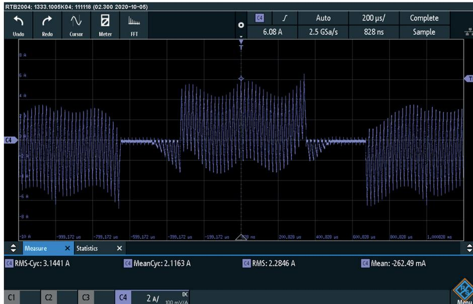
Figure 1: Phase Current Without Motor Choke
