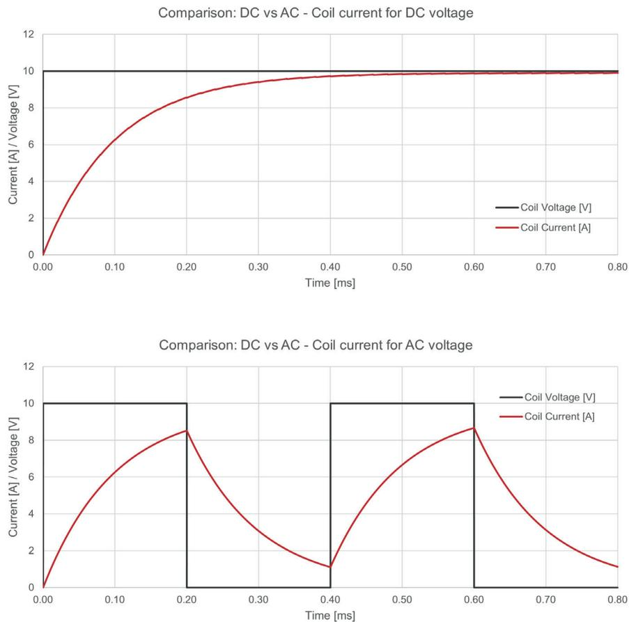
Figure 6: Current Behaviour Depending on Voltage Form
