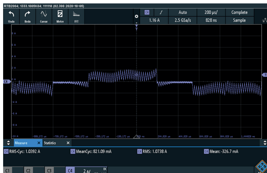
Figure 2: Phase Current With Motor Choke
