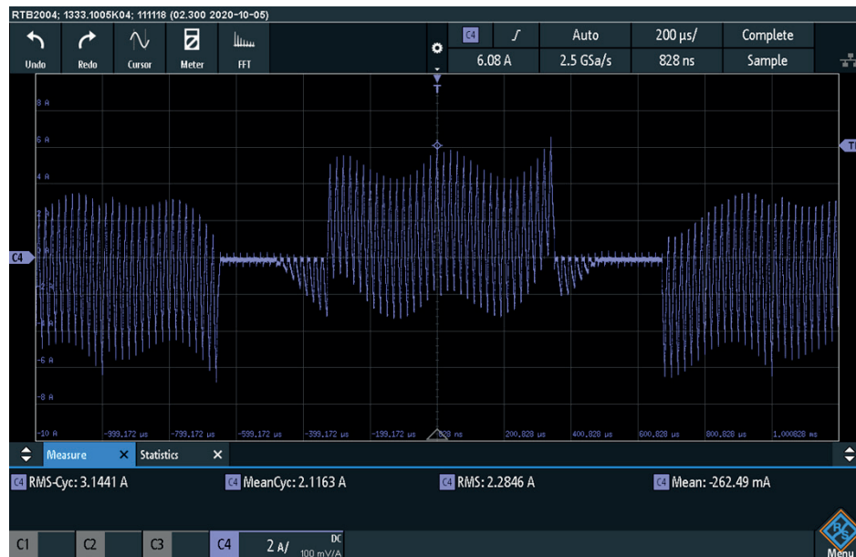
Figure 1: Phase Current Without Motor Choke
